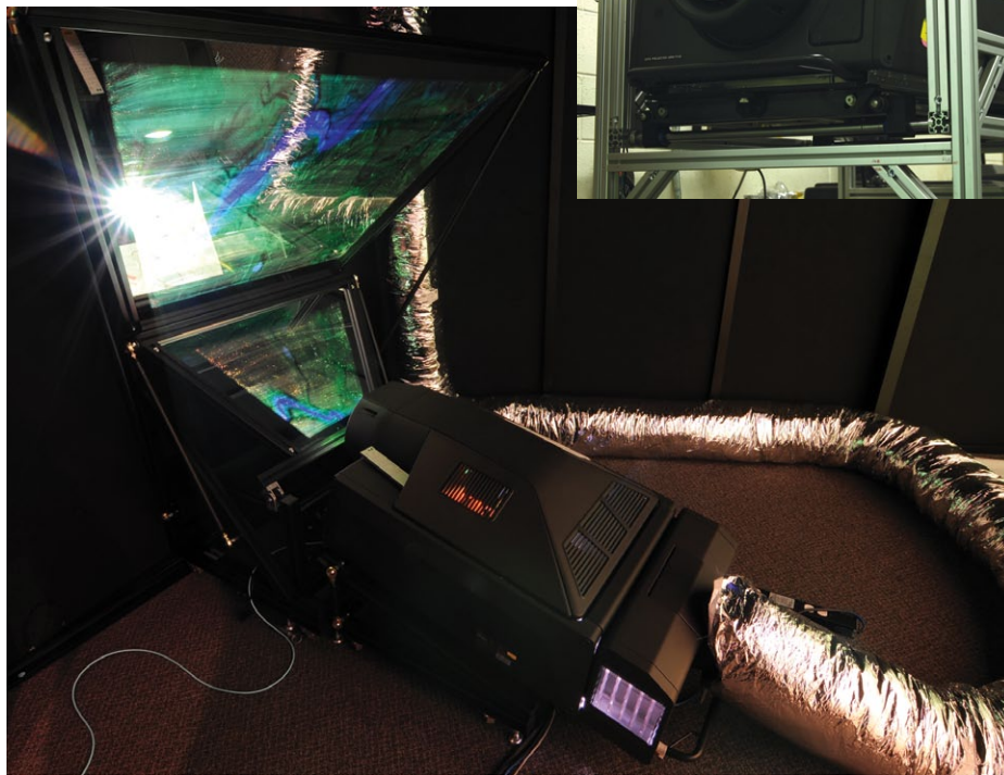
The 11,000 lumen 4K projector sits on a custom-built structure.
